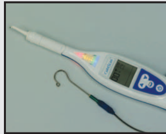
CarieScan Pro by CarieScan Occlusal lesion detection by AC impedance spectroscopy ( www.us.cariescan.com )
